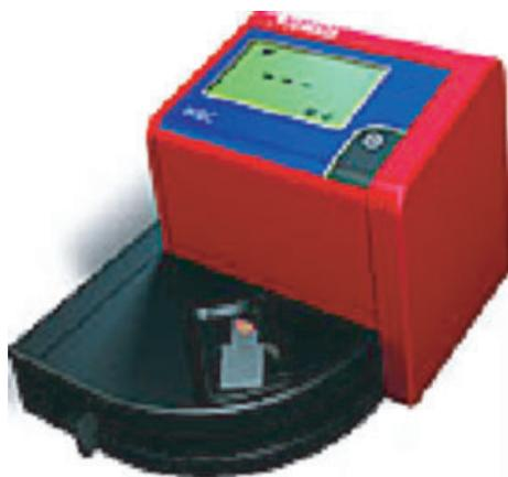
Figure 1. Photograph of the portable *HemoCue WBC* Point-of-care analyser (plastic cuvette containing a drop of blood is shown placed on the circular base holder).
